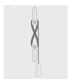
Breakaway safety tassel is pre-fitted to the lift cords so that when a horizontal force is applied to the cords entering the condenser it safely breaks away eliminating any hazardous loops.
