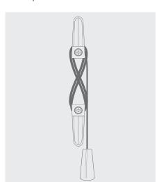
Breakaway safety tassel is pre-fitted to the lift cords so that when a horizontal force is applied to the cords entering the condenser it safely breaks away eliminating any hazardous loops.
