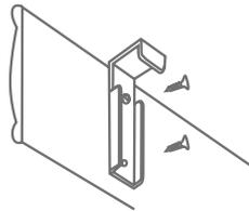
Hook valance clip with valance attached onto the top of the headrail.
